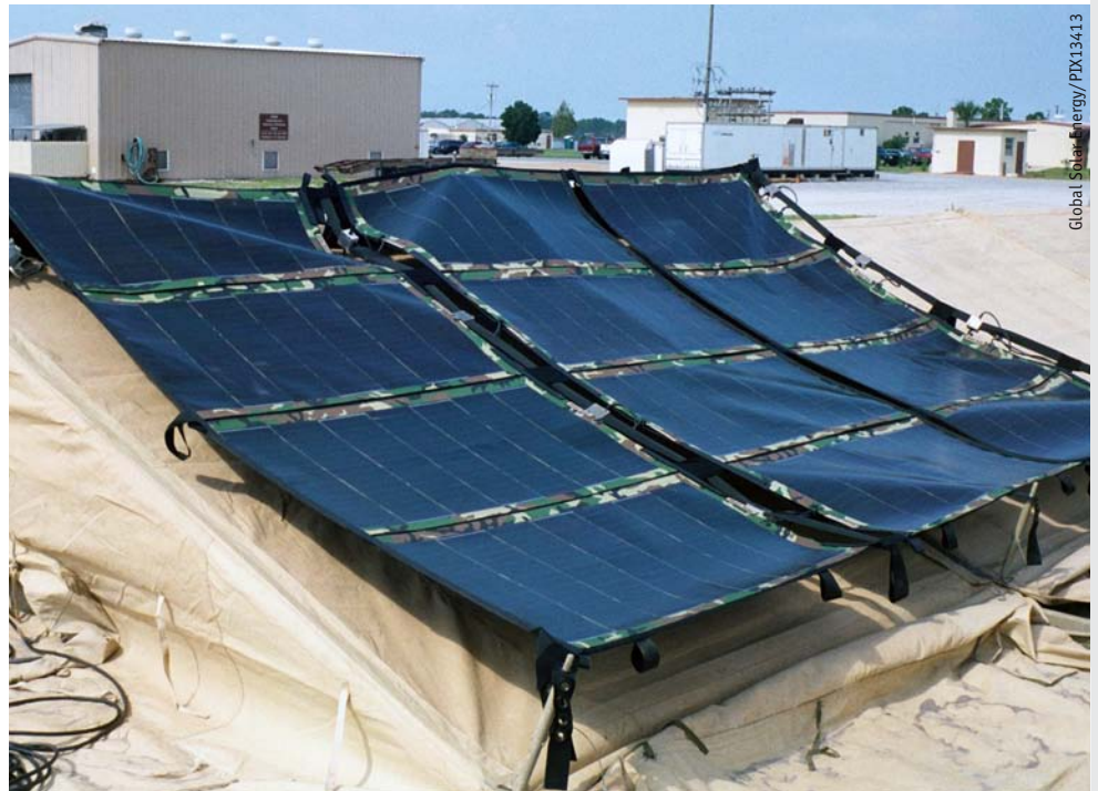
Thin-film copper indium gallium selenide (CIGS) PV creates a lightweight power supply that travels easily.
