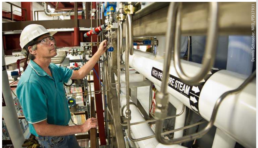
Master technician and pilot plant operator Robert Lyons inspects the high-solids pretreatment reactor in the Integrated Biorefinery Research Facility. The new reactor greatly enhances NREL's pretreatment testing and process development capabilities.
